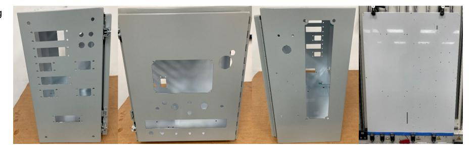
The ModCenter is also capable of cutting holes/penetrations in wire troughs and other steel/aluminum plates if the item fits within the machining "window" of the ModCenter.
